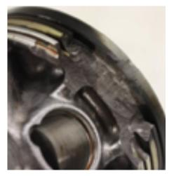
Two examples of piston damage due to LSPI (Source: www.infineuminsight.com)
